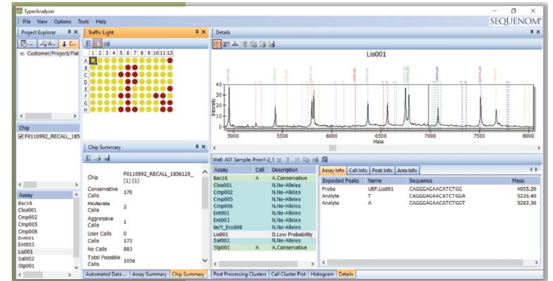
Figure 4 : TyperAnalyzer software for analysis of multiplexing reaction correlated to specific well on SpectroChip.
