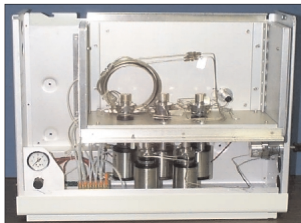
Figure 3: Inside view of valve oven layout.
