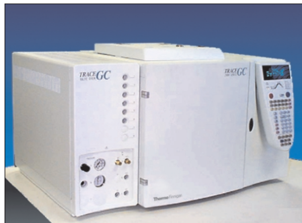
Figure 2: TRACE GC with optional valve oven
