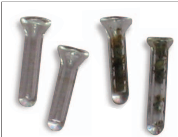
Figure 10: Direct Insertion Probe (DIP) tips. The crucibles on the left are new, while the crucibles on the right contain the non-volatile by-products of heating that were left over after analysis of the methamphetamine and cocaine powders.
