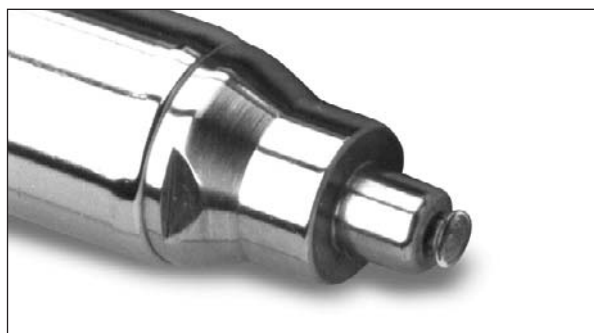
Figure 6: Insertion of the DIP crucible into the probe end. The crucible contains the powder sample.
