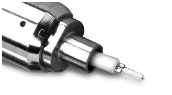
Figure 4: The direct insertion filament, shown with the loop on the end. A 1 \mu\text{L} sample is placed on the loop and the liquid allowed to evaporate prior to inserting the probe into the source.
