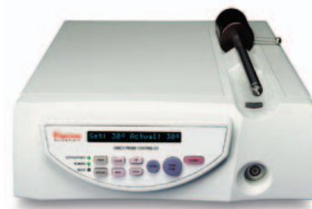
Figure 2: The Direct Sample Probe and controller. The keypad allows the User to enter method parameters and start and stop probe methods.
